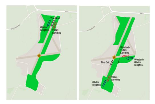
To make the best use of space on the runway, the first glider to arrive on each row should be positioned with its wingtip next to the grid marker, with the others behind it, as shown below.
